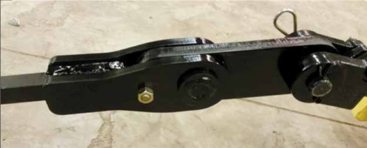
Shown above is the key link which attaches to the pulling cylinder on the right and a J-Link section on the left.
