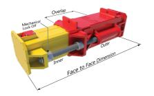
2500kN Hydraulic Strut assembly comprises inner and outer sleeved steel box sections housing a double acting (DA) hydraulic ram to provide up to 800mm of leg adjustment.
