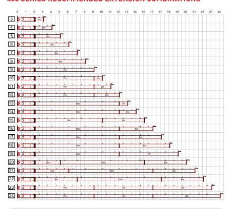
N.B. Single 0.25m and 0.5m extensions should be added to these combinations for intermediate dimensions. The strut assemblies are shown at mid-stroke, so each length can vary by up to 400mm in either direction.
